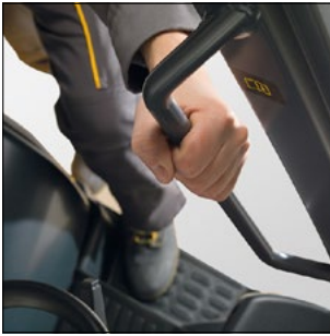
Entry via a deep, wide step. Large, strong grab handle welded to the overhead guard.
