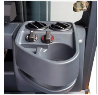
Heating including air demister for windscreen.
