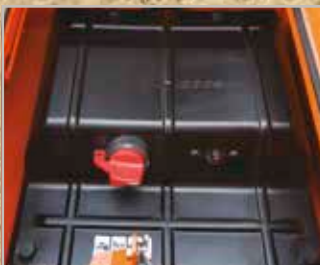
Battery cut-off switch
