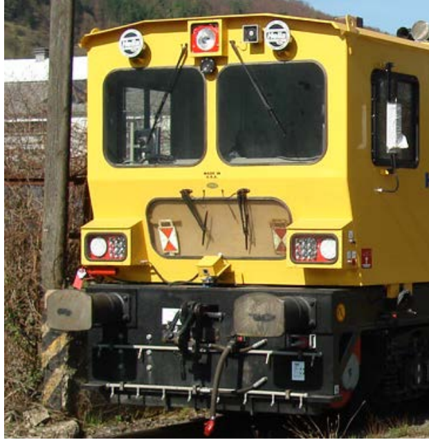
Front View of Similar Machine Showing Placement of Lights
