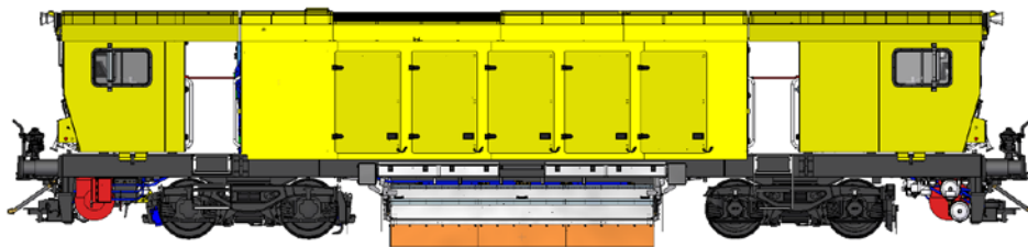
RGH10C2 Rail Grinder – 10-stone Machine Configuration
