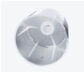
The non-genuine filter has a weaker ribbing, reinforcing only a part of the canister.
