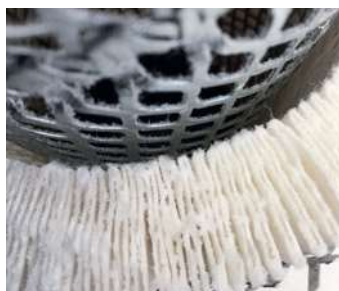
The non-genuine filter has a significant gap between the filter medium and the inner grid.
