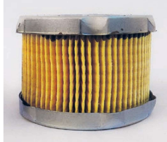
The non-genuine filter has a visible glue residue.
