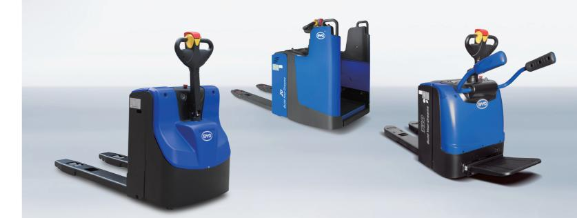
PTW20S is a pedestrian pallet truck with the rated capacity of 2000 kg, with compact design and standard with on-board charger.
