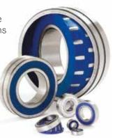
Solid Oil is an oil saturated, polymer material that virtually fills all of the free space in the bearing. In service, oil is released from the material into the narrow gaps between it and the bearing components, thus providing effective minimum quantity lubrication.
