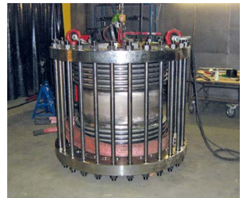
Testing a metal expansion joint with helium.
