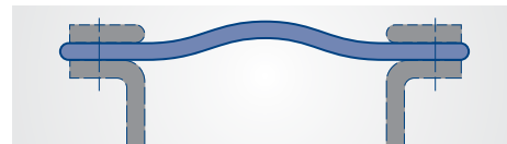
Flat belt expansion joint
