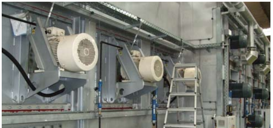
Continuous kilns' fan drives for the heat treatment of metal strips Photo by courtesy of Aurubis AG
